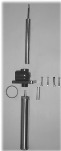
Instead of trying to resurrect the old pump, it can be converted into a modern Syphon Pump.
